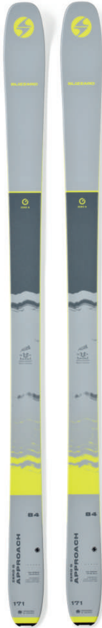
ZERO G 084 APPROACH (FLAT) COD: 8A1053 00 001 Lengths (cm) / Radius (m): 150/15, 157/16, 164/18, 171/19, 178/20, 185/22 Sidcut: 115-84-99 mm (171) Sug. binding: MARKER ALPINIST 12, MARKER KING PIN 13 Sug. skins: Skin Zero G 084 Approach Construction: Sandwich Compound Partial Sidewall (Carbon) Rocker: Rocker-Camber-Rocker Core + Key materials: Pawlonia Factory base bevel: 0.9° Factory side bevel: 87.7° Weight (flat): 1240 g (size 171)
