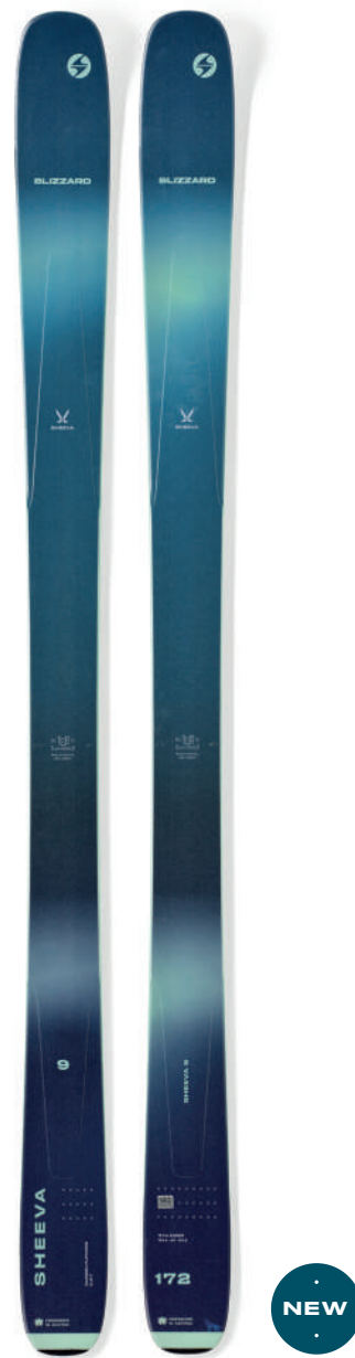
SHEEVA 9 (FLAT) COD: 8A2272 00 001 Lengths (cm) / Radius (m): 148/12.5, 157/13, 164/14, 172/15.5 Sidecut: 124-92-114 mm (164) Sug. binding: MARKER SQUIRE 11 ID - 110 Construction: Sandwich Compound Sidewall , Dynamic Release Technology Rocker: Rocker-Camber-Rocker Core + Key materials: Isocore, Poplar, Beech, Balsa, Poplania Factory base bevel: 0.9° Factory side bevel: 87.7° Weight (flat): 1790 g (size 164)
