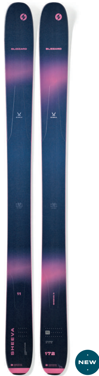
SHEEVA 11 (FLAT) COD: 8A2270 00 001 Lengths (cm) / Radius (m): 156/15, 164/16, 172/17.5, 180/19, 188/21 Sidecut: 139-112-129 mm (172) Sug. binding: MARKER GRIFFON 13 ID Construction: Sandwich Compound Sidewall , Dynamic Release Technology Rocker: Rocker-Camber-Rocker Core + Key materials: Isocore, Poplar, Beech, Balsa, Palwonla Factory base bevel: 1.3° Factory side bevel: 87.7° Weight (flat): 1880 g (size 172)
