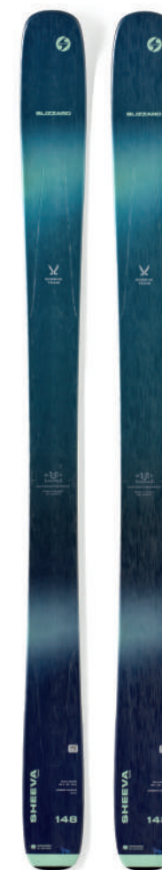
SHEEVA TEAM (FLAT) COD: 8A2273 00 001 Lengths (cm) / Radius (m): 140/11.5, 148/12.5, 156/13 Sidecut: 118.5-90-108.5 mm (148) Sug. binding: MARKER SQUIRE 10 - 100 Construction: Sandwich Compound Partial Sidewall , Dynamic Release Technology Rocker: Rocker-Camber-Rocker Core+Key materials: Poplar - Beech Factory base bevel: 0.9° Factory side bevel: 87.7° Weight (flat): 1230 g (size 148)
